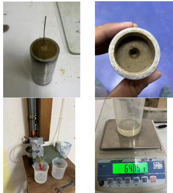
Figure 7 Pinhole test setup and sample preparation
