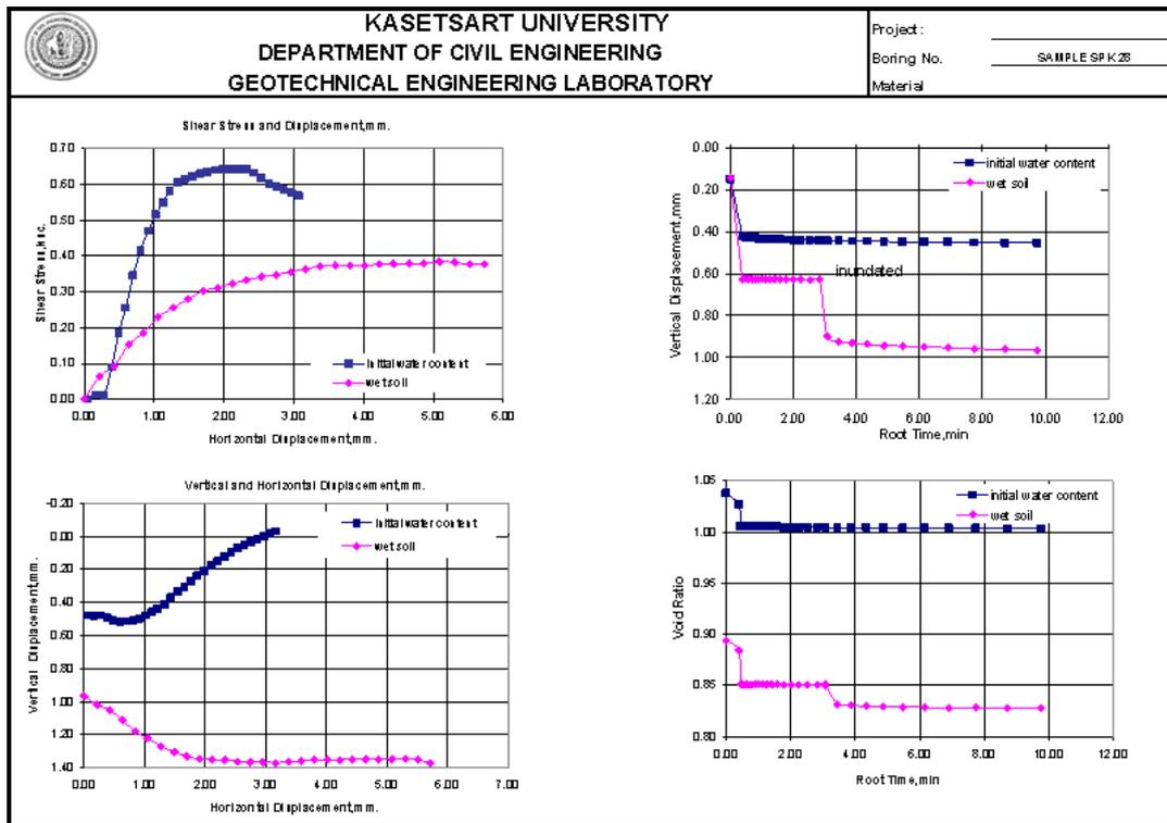
Figure 11 Example of the results of direct shear test for strength reduction index
