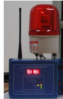
Fig. 14. Siren for landslide warning
