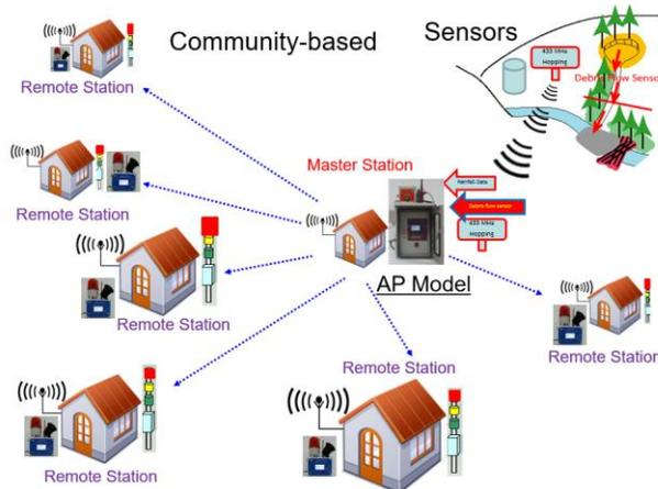
Fig. 13. Community based landslide warning system
