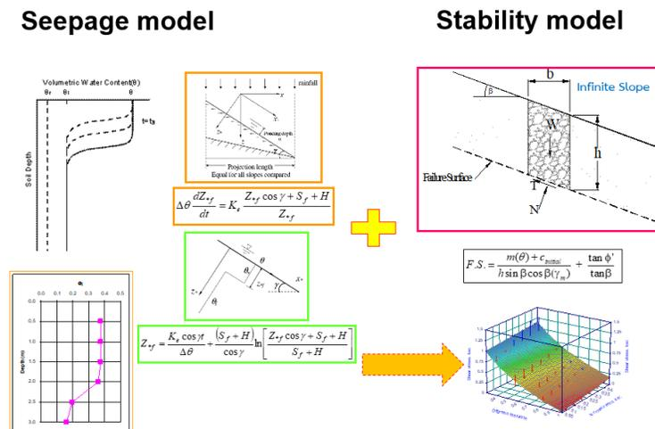
Fig. 11. Infiltration and Slope stability Analysis[19]
