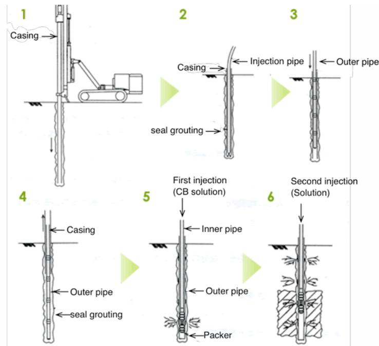
Fig. 5 Schematic view on double pipe and double packer methods
