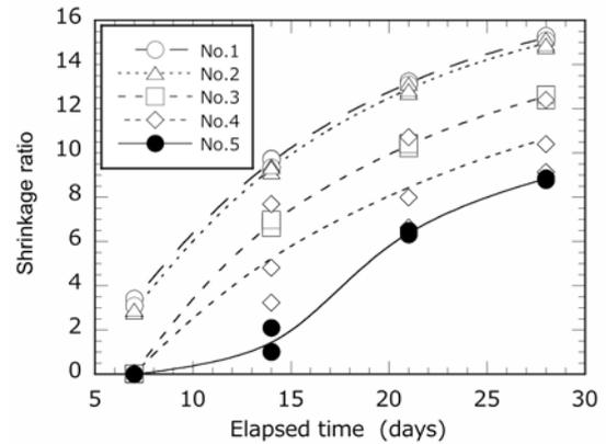
Fig. 11 Time series variation in shrinkage ratio of the homo-gel specimens mixed with liquid glass grouting agents with each molar ratio
