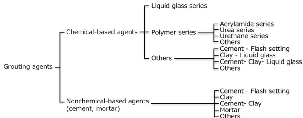
Fig. 1 Classification of grouting agents in chemical grouting techniques
