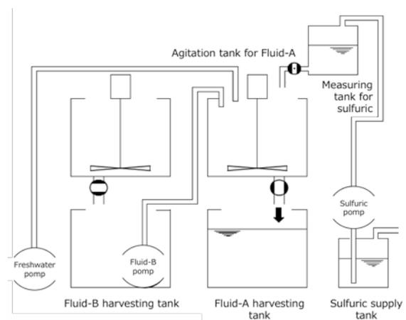
Fig. 9 Outline of the machine preparing injection fluid automatically
