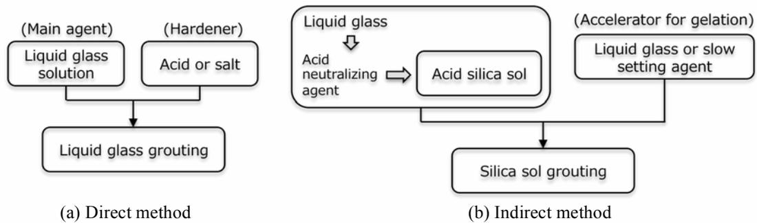
Fig. 8 Simple overview on mixing main agent and hardener during injection in direct and indirect methods
