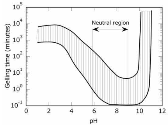
Fig. 2 Relationship between pH and gelling-time on the No. 5 liquid glass grouting agents
