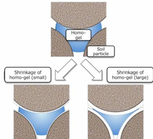
Fig. 12 Simple image on liquid glass grouting agents in voids of soil particles
