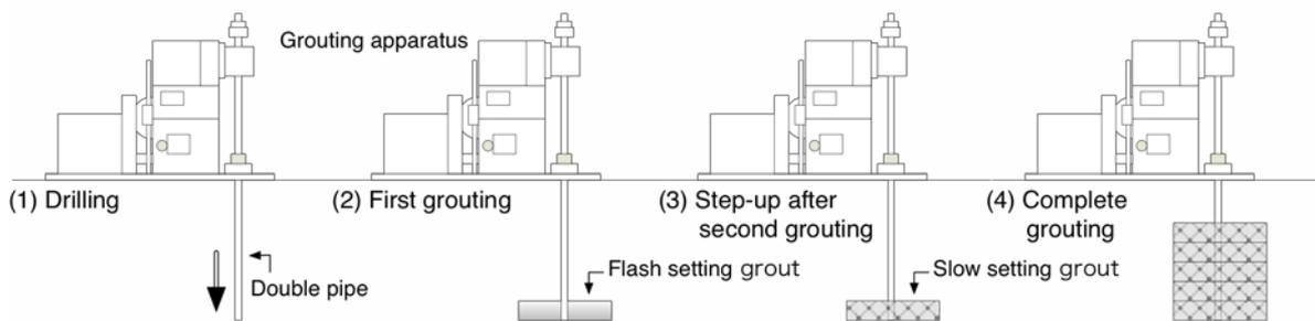
Fig. 6 Schematic view on double pipe strainer methods (diploid-phase)
