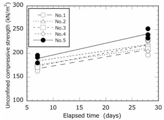
Fig. 10 Time series variation in unconfined compressive strength of the sand-gel specimens mixed with liquid glass grouting agents with each molar ratio
