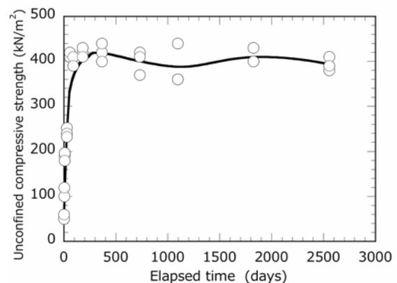
Fig. 4 Time series variation in unconfined compressive strength of the sand-gel specimen by the No. 5 liquid glass grouting agents
