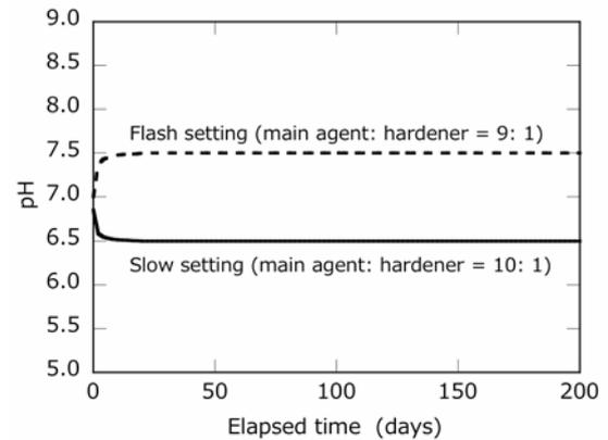
Fig. 3 Fluctuation of the immersion water pH from the sand-gel improved by the No. 5 liquid glass grouting agents
