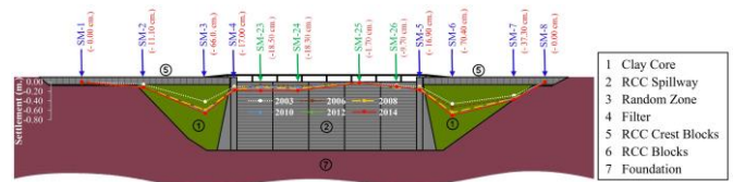
Figure 6 The settlement of the RCC section and earth fill (2014)
