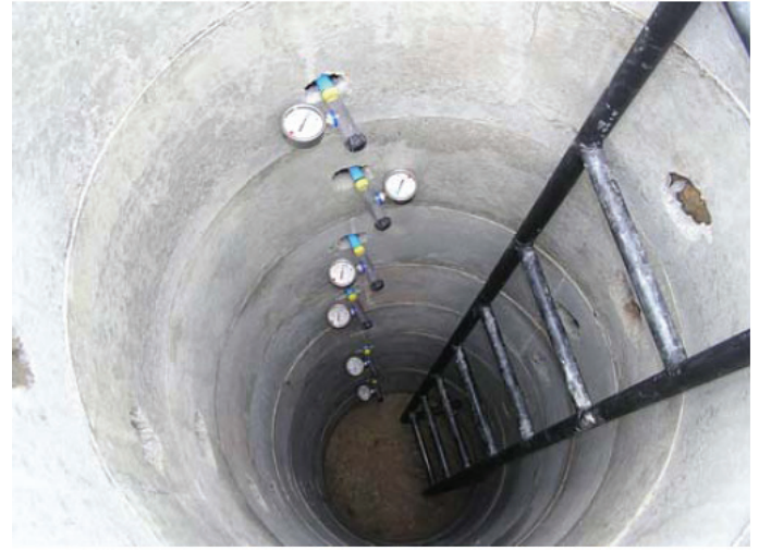
Figure 7: Tensiometer installation. (Mairaing et al., 2006).
