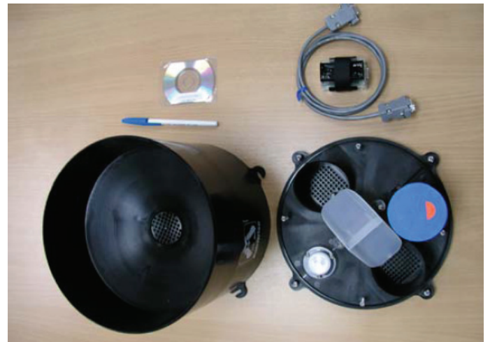
Figure 8: Automatic rain gauge. (Mairaing et al., 2006).
