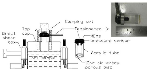
Figure 1: KU-tensiometer and its incorporation in direct shear box (modified from Jotisankasa and Mairaing, 2010).
