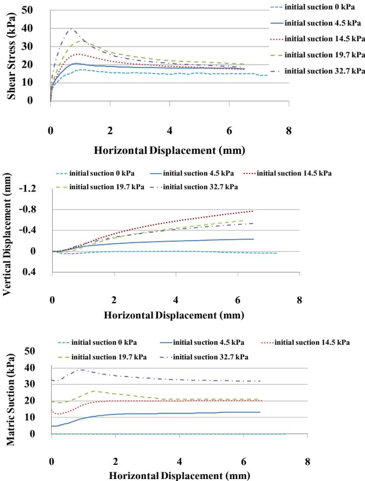
Figure 4: Typical results during constant-water content shearing in suction-monitored direct shear test on a compacted decomposed granite mixed with 20% kaolin.
