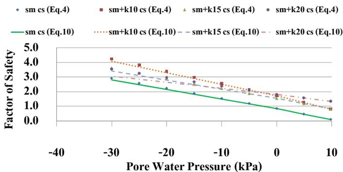
Figure 12: Variation between factors of safety and pore water pressure.
