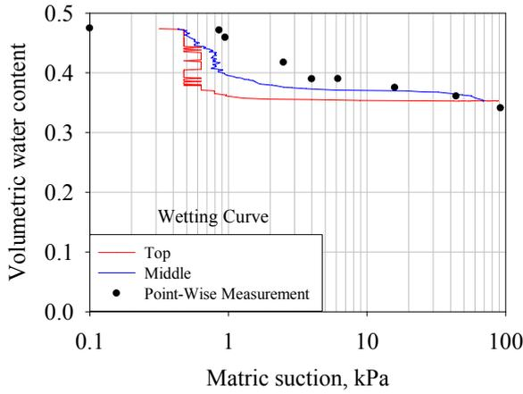
Figure 10: Wetting SWCCs from continuous measurement and point-wise measurement of a silty residual soil.
