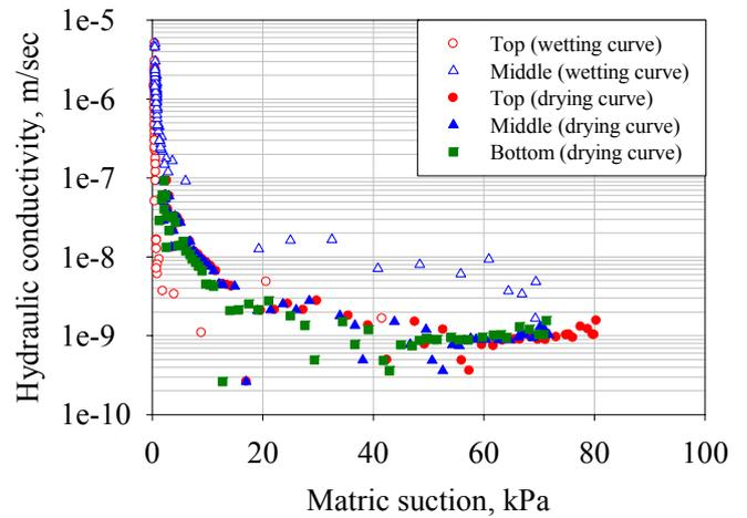
Figure 11: Permeability functions determined from continuous SWCC measurement.
