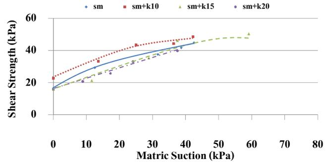
Figure 5: Peak shear strength versus matric suction envelope of decomposed granite (SM) mixed with different percentages of kaolin (0, 10, 15, 20% by weight) at normal stress of 15.5 kPa.
