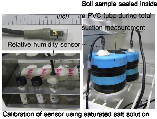
Figure 3: Relative humidity sensor, its calibration and its use for total suction measurement.
