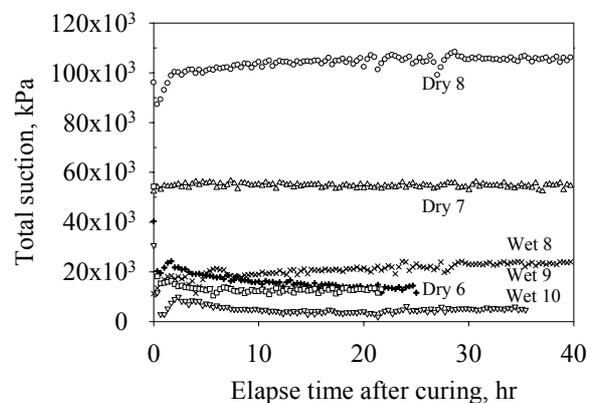
Figure 2: Typical results during measurement of (a) matric suction using tensiometer; (b) total suction using a relative humidity sensor (Tapparnich, 2010).
