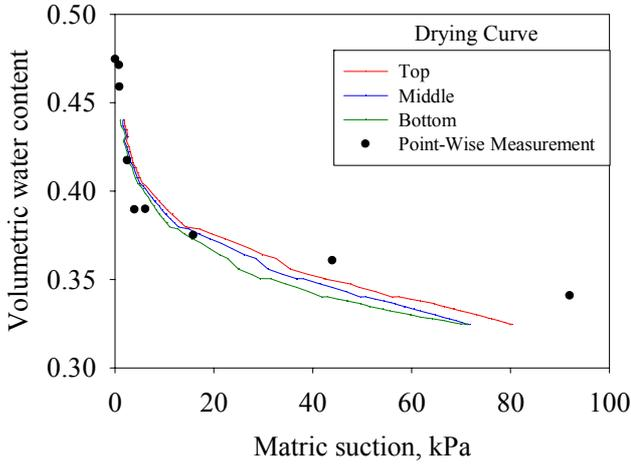
Figure 8: Drying SWCCs from continuous and point-wise measurement methods of a silty residual soil
