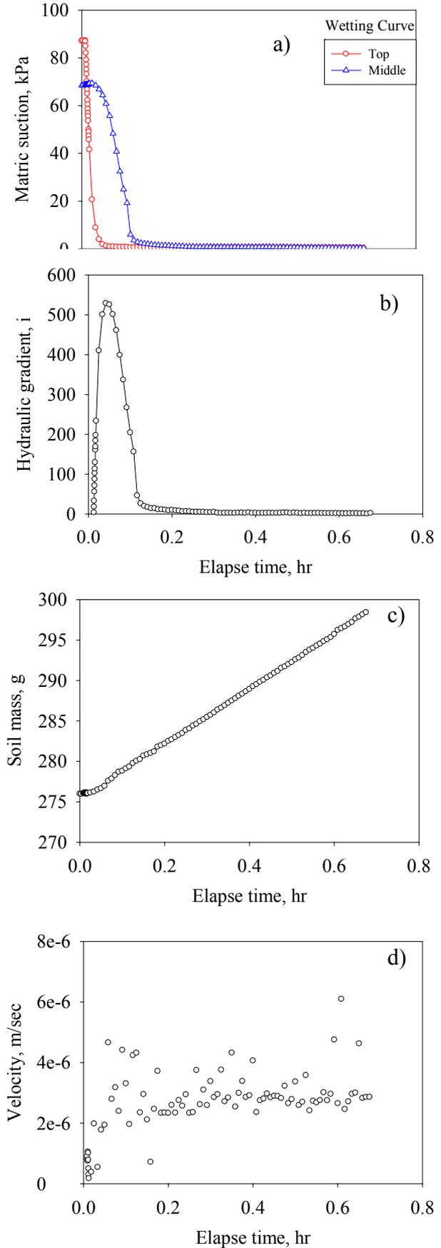
Figure 9: Typical results during wetting path of continuous SWCC measurement of a silty residual soil.
