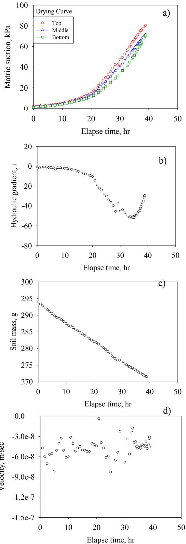
Figure 7: Typical results during drying path of continuous SWCC measurement of a silty residual soil.
