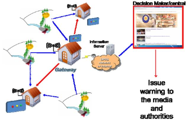
Fig.5: Multi-way landslide and debris flow prediction and warning concept.
