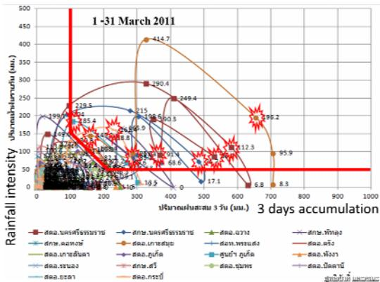
Fig.3: Landslide and debris flow warning curve based on statistical data.
