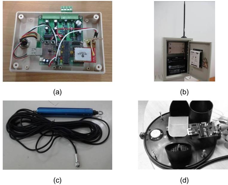
Figure 3 Wireless sensor node and sensor devices: (a) inside a unit showing a microcontroller and a high-power RF transceiver, (b) an enclosure with an 18Ah battery and an external antenna, (c) a debris flow detector, and (d) tipping bucket rain gauge
