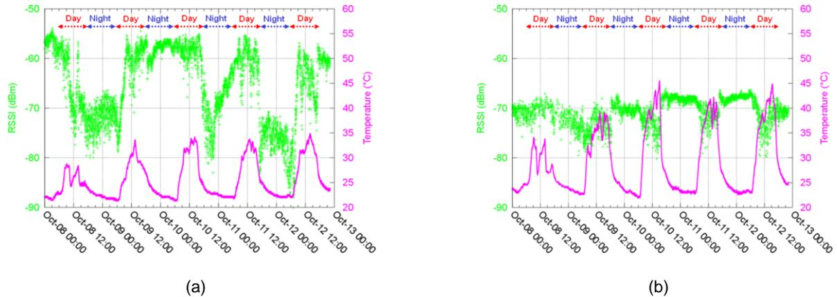
Figure 8 Records of signal strengths and temperature data: (a) bushy area, and (b) clear area
