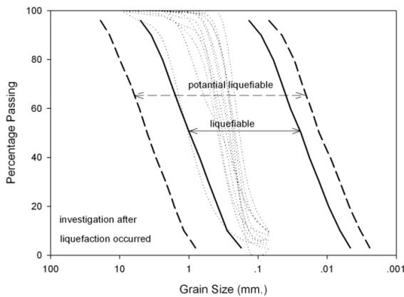
(b) Gradation curve of extruded liquefied sands collected on the ground surface after liquefaction occurred
