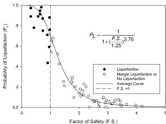
Figure 8 : Probability of liquefaction variation with liquefied FS for CSR approach in Maesai region
