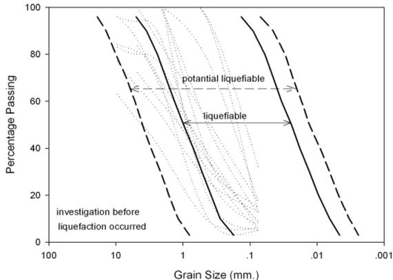
(a) Gradation curve of soil in sand layers collected before earthquake
