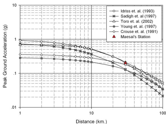
Figure 2 : Attenuation relationship comparing with recorded peak acceleration at Maesai's station
