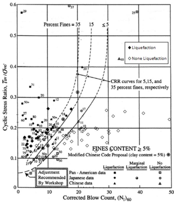
Figure 7 : Liquefaction potential of Maesai from Tarlay Earthquake 2011 plotted in Seed's curve
