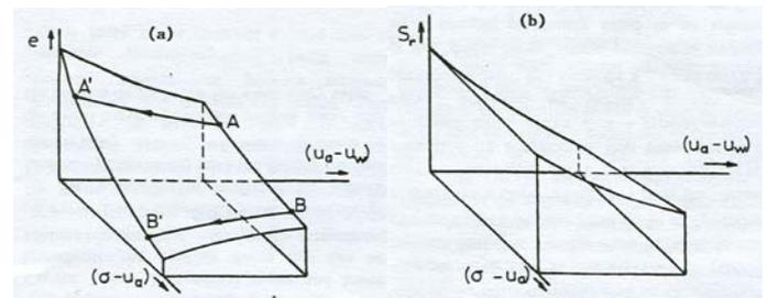
**Figure 5** State surface concept for void ratio and degree of saturation, Wheeler & Karube [15]
