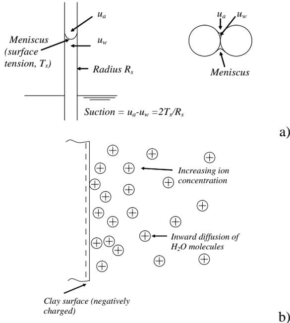
**Figure 1** The two phenomena contributing to the matrix suction; a) capillarity; and b) water adsorptions by a clay particle surface.
