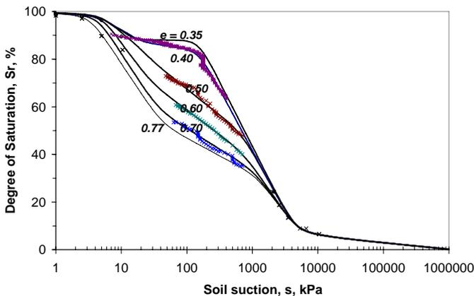
**Figure 3** Contours of the main wetting surface for the compacted silty clay. The symbols indicate the processed data, Jotisankasa [11].
