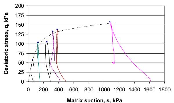
**Figure 7** Results for unconfined compression tests on the Saprolitic sandy clay from Nam-Kor landslide
