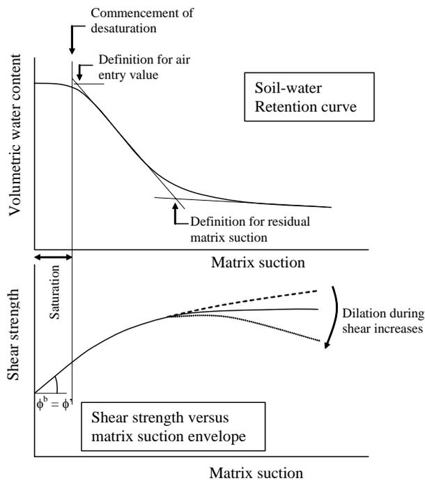
**Figure 4** Schematic relationship between soil-water retention curve and shear strength versus matrix suction envelope, Gan & Fredlund, [18]
