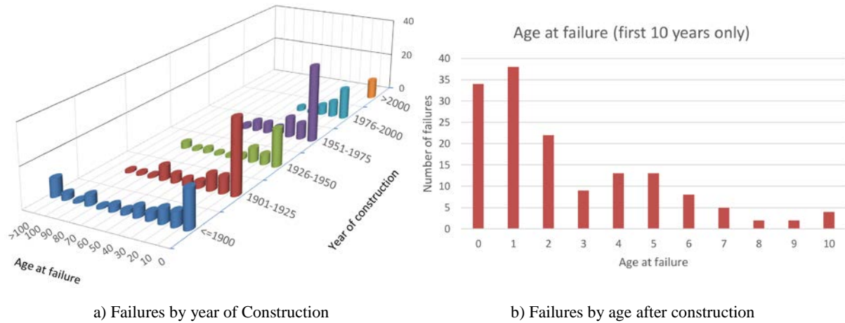
Figure 3 Distribution of Failures by Periods of construction and age after construction
