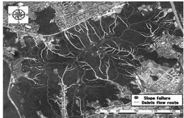
Figure 3. Locations of Slope Failures and Debris Flows around Umyeon Mountain in 2011
