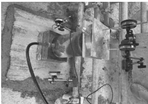
Figure 2. Typical set-up for pull-out tests.
