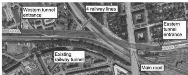
Figure 1. Horizontal alignment and key structures.
