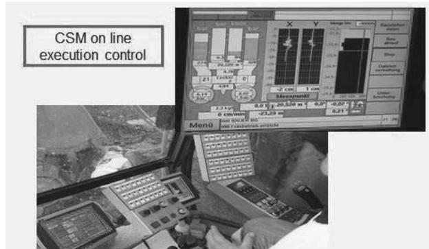
Figure 5. CSM on line execution control.
