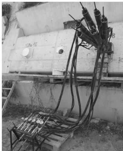
Figure 2. Test setup for simultaneous stressing of all strands of prestressed ground anchors using monostrand jacks.
