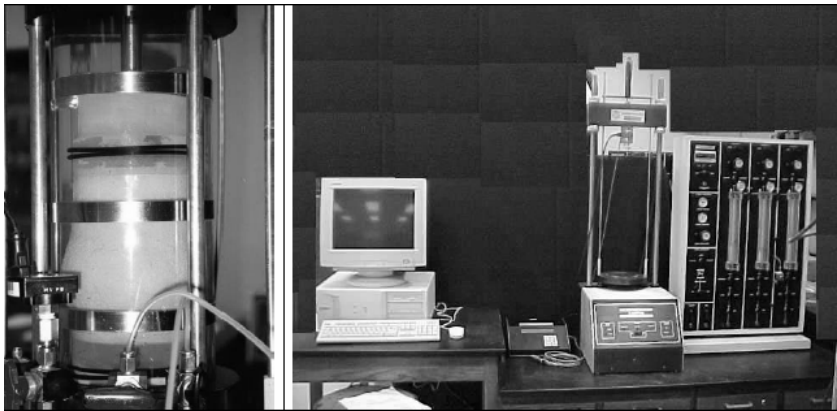
Load frame, pressure panel, and computerized data acquisition system
